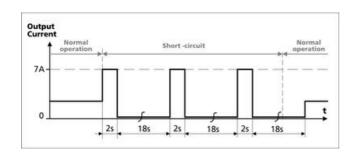
Thanks to the unique Pul Hiccup<sup>plus</sup> ensures a high short circuit current while avoiding the risk of overheated cables and damage to the connected loads. When a short circuit occurs following.
